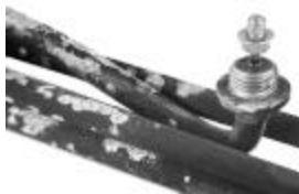
RUST BUILD-UP ON ELEMENT
