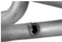
SHEATH BURNED- OUT DUE TO DRY FIRE
